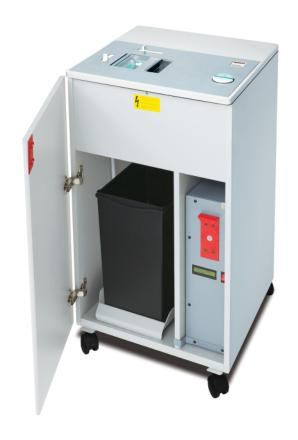
Comprehensive SPS safety package (HDP unit): Easy Switch control element uses illuminated color codes and symbols to indicate operational status and functions as an emergency stop switch; electronically controlled, transparent safety shield in the feed opening; automatic stop after punching; automatic power cut-off when cabinet is opened or collection bin is full; double protection against overheating.
